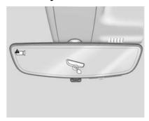
See your dealer for service if a blue screen and are displayed in the mirror, and the display shuts off. Also, push the tab as indicated to return to the automatic dimming mode.
