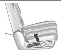
2. Lift the lever on the outboard side of the seat to release the seatback.
