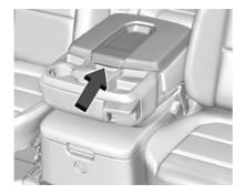
If equipped, pull the front center armrest down to access the storage area with cupholders.
