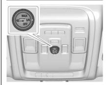
If equipped, the power liftgate switch is on the overhead console. The vehicle must be in P (Park).
