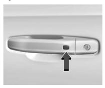
The remote key must be within 1 m (3 ft) of the liftgate or door being opened or locked. Press the button on the door handle to open. See "Keyless Access Operation" in Remote Keyless Entry (RKE) System Operation
