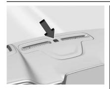
There is a light sensor on top of the instrument panel. Do not cover the sensor, otherwise the headlamps will come on when they are not needed.
