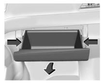
Press the sides of the glove box bin inward to clear the stoppers and rotate downward to lower the bin.
