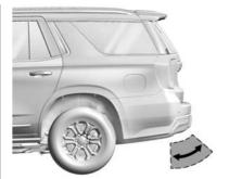
To operate, move your foot in a forward kicking motion under the center of the rear bumper, then pull it back.
