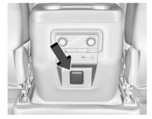
When the ignition is on, power to the 110 Volt outlet is enabled after the Substantial button is pressed, see *Instrument Panel Overview* \$\dip 4\$ for button location. A green indicator light on the button indicates when the 110 Volt outlet is enabled. 110 Volt power is supplied to the outlet when it is enabled and electrical equipment is plugged into that outlet. One power outlet can be
