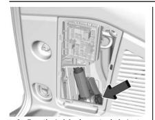
2. Turn the jack knob counterclockwise to release the jack and wheel blocks from the bracket. If equipped, remove the wheel blocks from the jack and place the wheel blocks on both sides of the tire at the opposite corner of the tire being changed. See If a Tire Goes Flat ⇒ 345 for more information on the placement of the wheel blocks. Place the jack and wheel blocks near the tire being changed.
