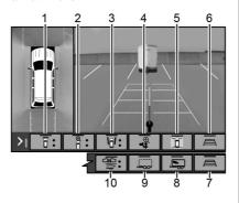
Touch the camera view buttons along the bottom of the infotainment display to access each view (if equipped):
