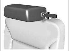
The head restraint will fold forward automatically.
