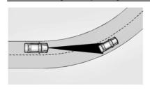
ACC may detect a vehicle that is not in your lane and apply the brakes.
