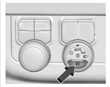
If equipped with fog lamps, the button is on the exterior lamp control, to the left of the steering column. The ignition must be on for the fog lamps to come on.
