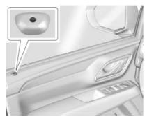
A light on the upper surface of the driver's door trim is used to indicate vehicle security status.
