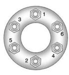
Tighten the nuts firmly in a crisscross sequence as shown by turning the wheel wrench clockwise.
