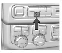
Press at to enable or disable HDC. Vehicle speed must be below 60 km/h (37 mph).
