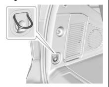
There are two cargo tie-downs in the rear cargo area. These can be used to strap cargo down and keep it from moving inside the vehicle.
