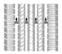
Treadwear indicators are one way to tell when it is time for new tires. Treadwear indicators appear when the tires have only 1.6 mm (1/16 in) or less of tread remaining. See *Tire Inspection* \$ 339 and *Tire Rotation* \$ 339 for additional information.
