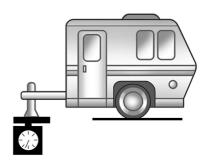
The Maximum Trailer Tongue Weight Rating for a conventional trailer hitch is shown on the Trailering Information Label.
