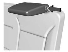
The head restraint will fold forward automatically.
