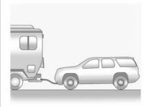
Only dinghy tow four-wheel-drive vehicles with a two speed transfer case that has an N (Neutral) and a 44 setting.
