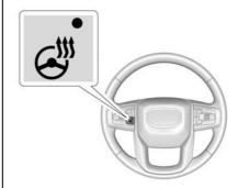
: If equipped, press to turn the heated steering wheel on or off. An indicator next to the button is lit when the feature is turned on.
