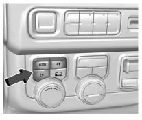
If equipped, the transfer case controls are used to shift into and out of four-wheel drive.
