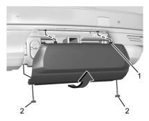
To remove hitch cover, if equipped:
