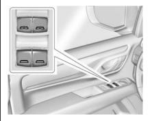
The power windows work when the ignition is on, in ACC/ACCESSORY, or when Retained Accessory Power (RAP) is active. See Retained Accessory Power (RAP) ⇒ 208.
