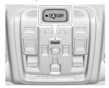
There are dome lamps in the overhead console and the headliner.
