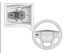
S: Press to turn cruise control on or off. A white indicator comes on or off in the instrument cluster.
