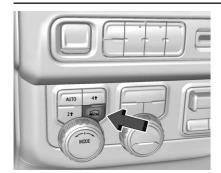
If equipped, select Terrain Mode by pressing the below the 4 1 transfer case button.
