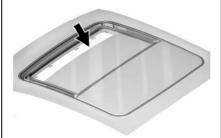
Dirt and debris may collect on the sunroof seal or in the track. This could cause an issue with sunroof operation or noise. It could also plug the water drainage system. Periodically open the sunroof and remove any obstacles or loose debris. Wipe the sunroof seal and roof sealing area using a clean cloth, mild soap, and water. Do not remove grease from the sunroof.
