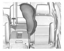
If the vehicle has a front center airbag, it is in the inboard side of the driver seatback.
