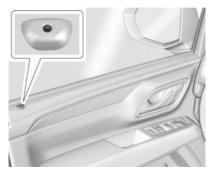
The indicator light, on the driver door near the window, indicates the status of the system. See *Power Door Locks*
