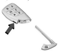
Press the button on the side of the remote key and pull the mechanical key out. Never pull the mechanical key out without pressing the button.
